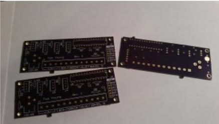
Doing some continuity checks before I begin soldering and risk blowing components up
