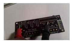
Most parts are on, save the I2C resistors and the heat sinks. Time to program the microcontroller:
