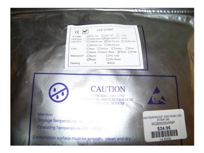
It's a 5 meter strip of 5050 RGB LEDs, on a spool, covered in waterproof resin. You can cut them every 3 LEDs (50mm) and the strip has a self-adhesive backing. Seems perfect for cabinets!
