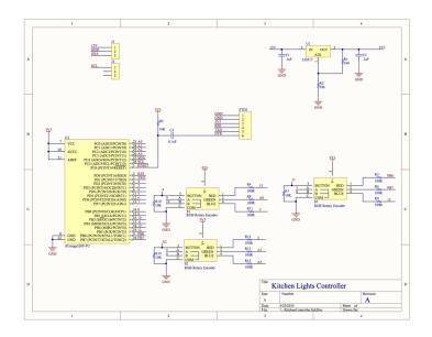
Okay, the schematic is done! Let's turn this into a printed circuit board (PCB). I need this to fit inside an outlet box. I measured mine at 3" x 1.5" for a not-too-snug fit.
