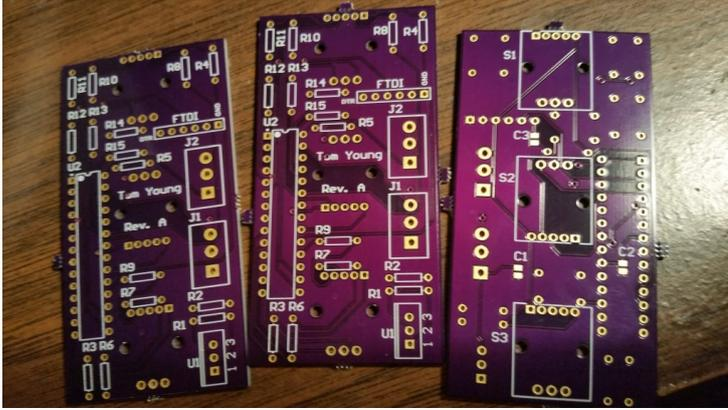
Looks like I forgot to label the ports on the silkscreen for the screw terminals. Oh well. I started soldering almost immediately. Some top components:
