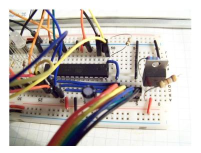
I set the fuses for the 8MHz Internal RC oscillator and pushed the following command to get the chip running. avrdude -p m328p -P /dev/cu.usbmodem142411 -c avrisp -b 19200 -U lfuse:w:0xe2:m -U hfuse:w:0xda:m -U flash:w:ATmegaBOOT\_168\_atmega328\_pro\_8MHz.hex
