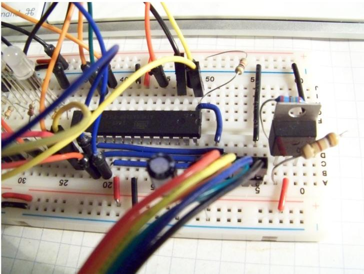
I set the fuses for the 8MHz Internal RC oscillator and pushed the following command to get the chip running.
