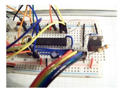
I set the fuses for the 8MHz Internal RC oscillator and pushed the following command to get the chip running. avrdude -p m328p -P /dev/cu.usbmodem142411 -c avrisp -b 19200 -U lfuse:w:0xe2:m -U hfuse:w:0xda:m -U flash:w:ATmegaBOOT\_168\_atmega328\_pro\_8MHz.hex
